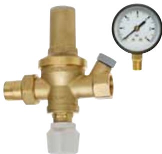
Art. 249 + Art. 244 Heavy model filling group with stop cock and filter. 1/4" connection for gauge. Check valve. Max. inlet pressure 20 bar, adjustable outlet pressure from 1 to 6 bar (factory setting 1,5 bar), max. working temperature 90°C. With gauge.
